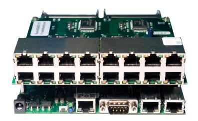
The new RB816 is an expansion board for RouterBOARD 800 and also the RouterBOARD 600 series. It attaches to the RouterBoard device to add 16 additional 10/100 ethernet ports.
